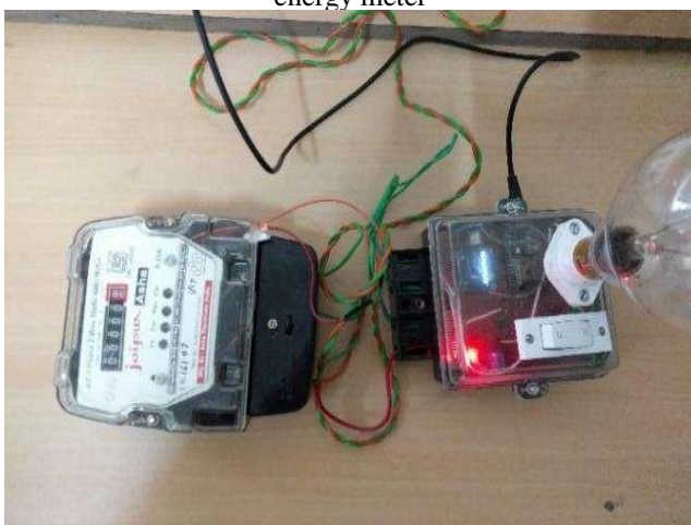
Figure 8. Experimental setup of IoT based smart energy meter in laboratory
